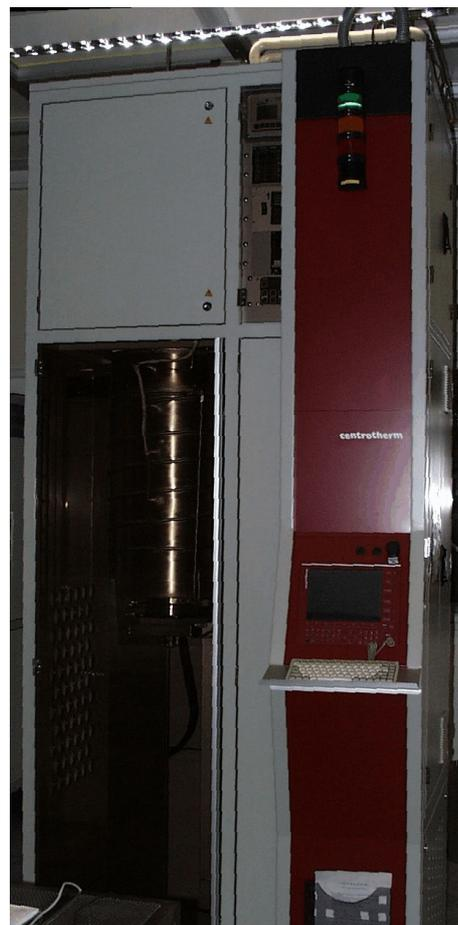
Fig. 1: Vertikales Hochtemperaturofensystem; Vertical high-temperature furnace system.
