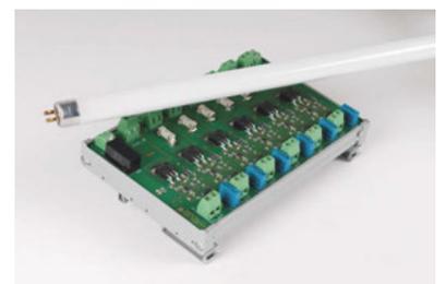
17) HV-DC switch board for office light control: six channels each 380 V / 1 A for 6x 50 W fluorescent lamps (DIN rail mounting); suitable for capacitive inrush
