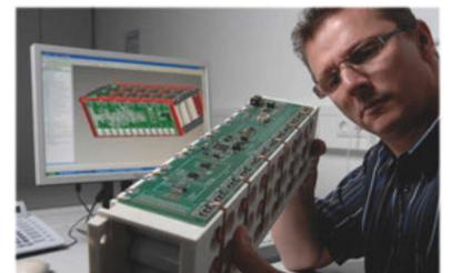
24) Full-custom battery system design, including mechanical, thermal and electrical engineering
