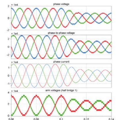
10) Numerical circuit simulation of a modular multi-level converter
