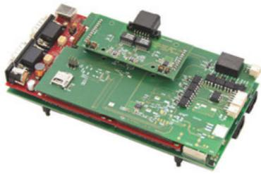
28) Highly modular battery management system (BMS) for mobile and stationary applications. Photo shows the safety and monitoring control boards with their analog and digital interfaces
