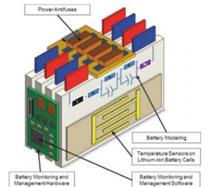
25) Research and development topics in the fields of battery system design, sensor and actuator developments for battery systems at Fraunhofer IISB
