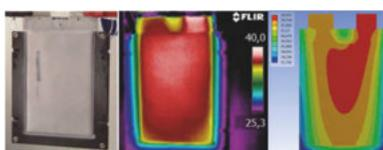
31) Highly-accurate coupled electro-thermal modelling, simulation and characterization of battery cells and complete systems
