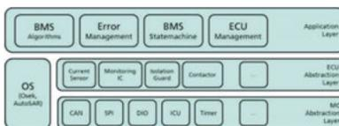
30) Software engineering for the battery management system (BMS), including battery state computation algorithms (SOC, SOH, SOL, SOF) and safety
