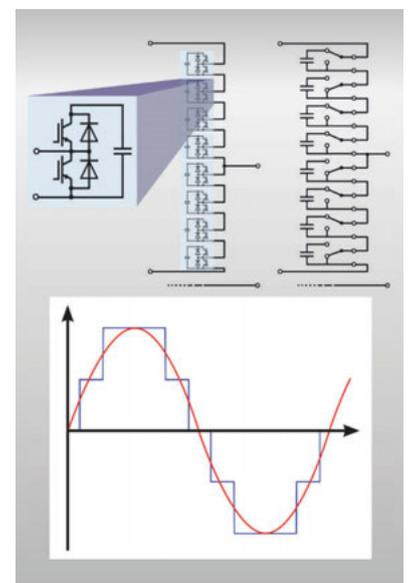
9) Basic principle of a modular multi-level converter (M2C)
