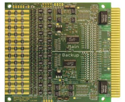
26) High-end daisy chainable universal battery monitoring electronics with full redundancy for safety-critical high-availability applications offering up to  $\pm 1.2\text{mV}$  accurate cell voltage measurement, NTC-based or sensorless temperature measurement, active or passive balancing with balancing status monitoring
