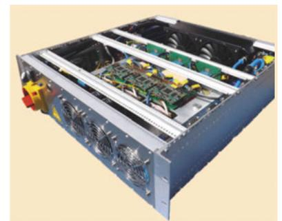
16) Bidirectional isolating DC/AC bridge (3.7 kW) with two DC/DC channels for MPP tracking of PV strings (3.7 kW) and one bidirectional DC/DC channel (7.4 kW) for the management of a stationary battery
