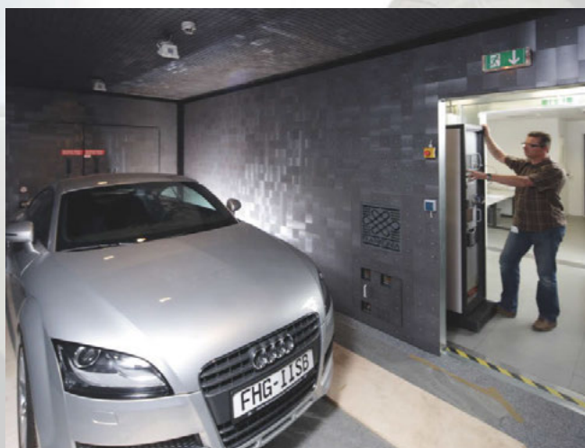
EMC test chamber for pre-compliance measurements
