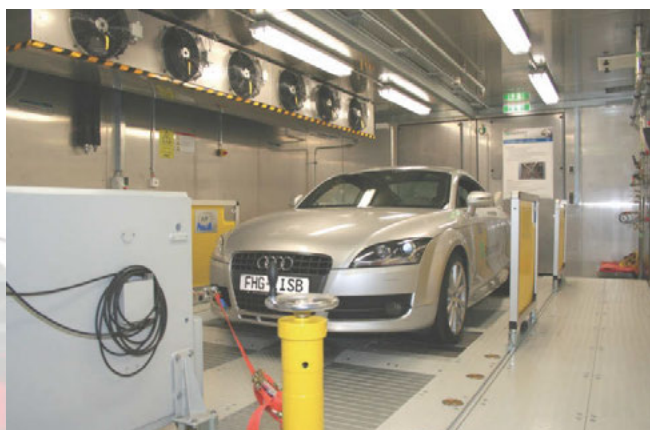
The 4-WD dynamometer (4x 85 kW) in the vehicle test center
