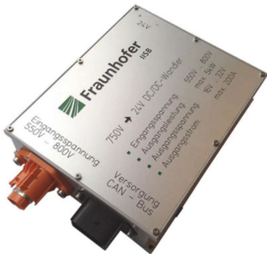
Insulating 5 kW DC/DC converter from 750 V to 24 V for trucks
