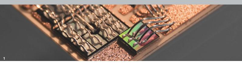
1 Snubber device for power electronic converters
