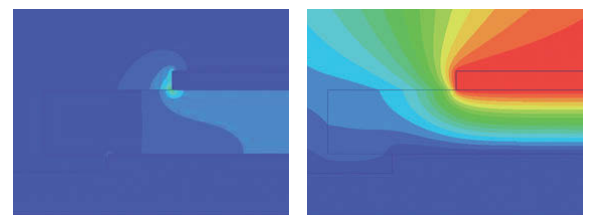
Metal-ceramic-metal structure with a voltage load on the upper metallization, the potential distribution and the electric field strength enhancement.
