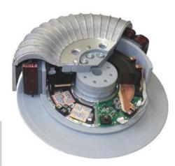
The picture shows an IGBT-inverter system completely integrated into the stator of a 6-phase wheel-hub-motor. Available space was about 2 liters. The external-rotor PMSM has a continuous power of 30 kW and a peak-power of 65 kW at a nominal DC-link voltage of 400 V.
