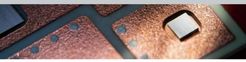
1 SiC MOSFETs embedded in DBC substrate with vias
