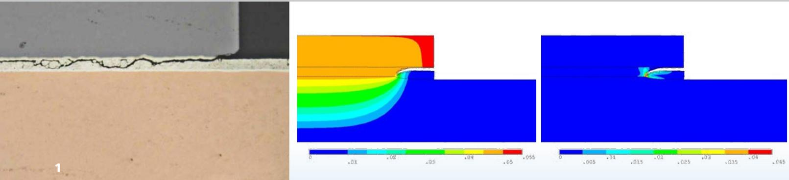
1 Crack propagation in sintered die-attachment layer. Left: Experiment, Center: Simulated deformation field, Right: Simulated stress field.
