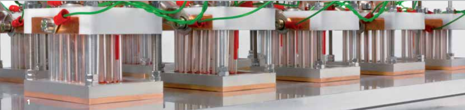
1 Thermal characterization of power modules mounted on a water-glycol cooled heat sink
