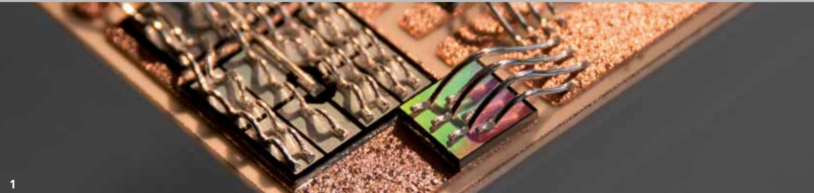
1 Snubber device for power electronic converters
