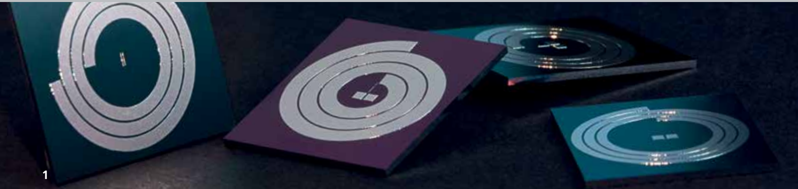
1 Diced planar-spiral inductors with air core and Al winding on Si-substrate
