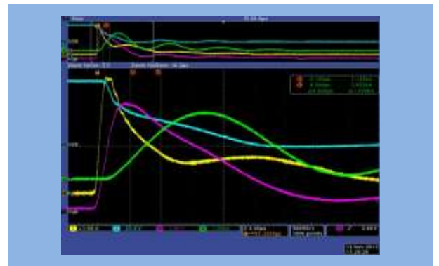
Switching behavior check on power semiconductors
