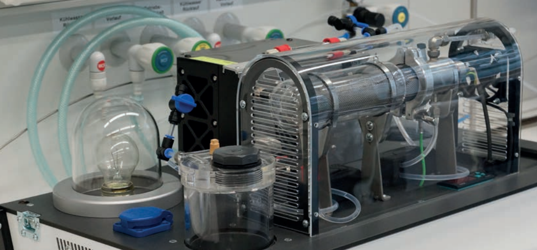
Compact demonstrator setup for the dehydrogenation of liquid organic hydrogen carriers
