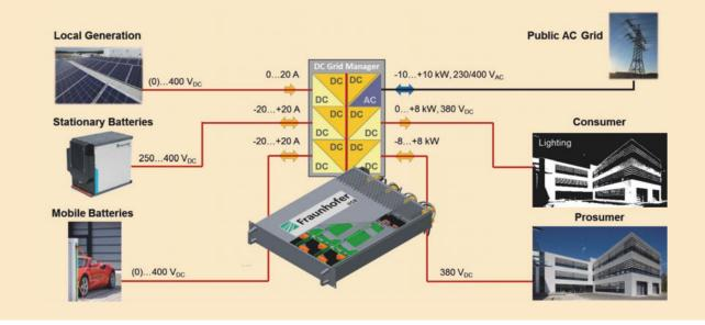
19) The universal DC grid manager – a system solution from Fraunhofer IISB
