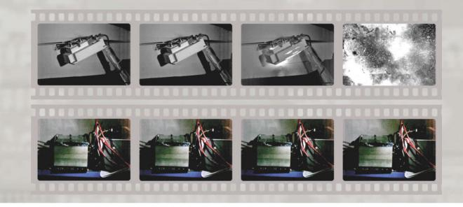
6) Experimental investigation of hazardous events with a high-speed camera. Top frame: 1.7 kV IGBT module without enclosure - debris damage converter system; Bottom frame: Hazard proof IISB solution debris fully captured
