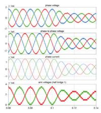
10) Numerical circuit simulation of a modular multi-level converter
