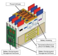
25) Research and development topics in the fields of battery system design, sensor and actuator developments for battery systems at Fraunhofer IISB
