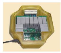
22) Drive inverter for direct motor attachment with an innovative cooling solution based on thermally enhanced polymers.
