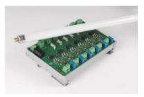
17) HV-DC switch board for office light control: six channels each 380 V/1 A for 6x 50 W fluorescent lamps (DIN rail mounting); suitable for capacitive inrush
