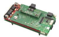
28) Highly modular battery management system (BMS) for mobile and stationary applications. Photo shows the safety and monitoring control boards with their analog and digital interfaces
