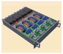
20) Rack mounted (19") multiport DC/DC converter (8 bidirectional channels each with 20 A; max. voltage 430 V, efficiency 99%); CAN interface
