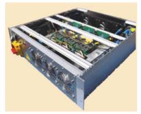
16) Bidirectional isolating DC/AC bridge (3.7 kW) with two DC/DC channels for MPP tracking of PV strings (3.7 kW) and one bidirectional DC/DC channel (7.4 kW) for the management of a stationary battery
