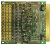
26) High-end daisy chainable universal battery monitoring electronics with full redundancy for safety-critical high-availability applications offering up to ±1.2mV accurate cell voltage measurement, NTC-based or sensorless temperature measurement, active or passive balancing with balancing status monitoring
