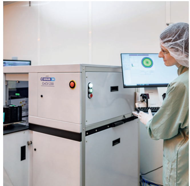
Corona non-contact CV measurements for doping uniformity. © Daniel Karmann / Fraunhofer IISB
