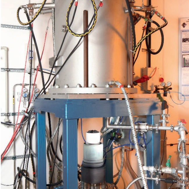
Lab furnace for directional solidification of silicon © Kurt Fuchs / Fraunhofer IISB
