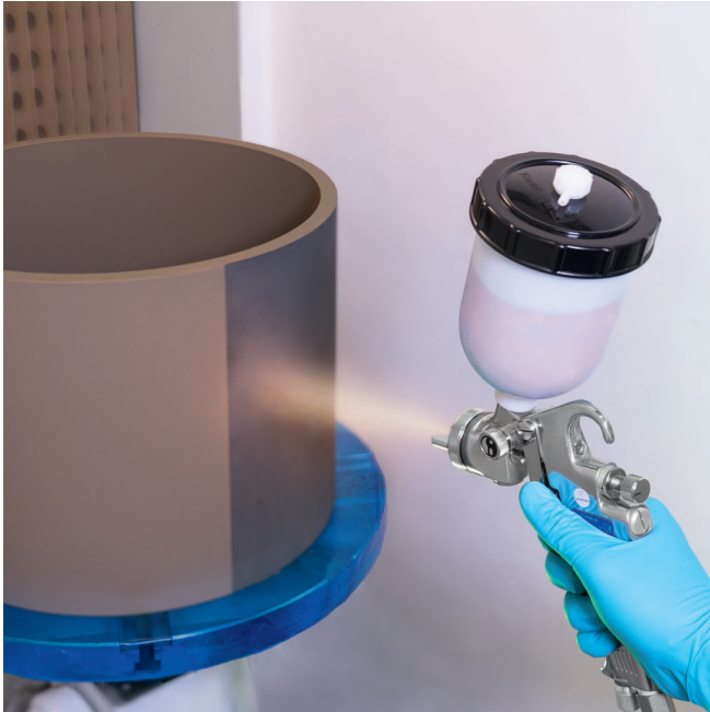
Spray coating of graphite parts with TaC © Elisabeth Iglhaut / Fraunhofer IISB
