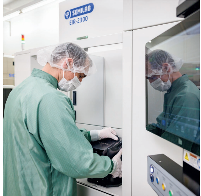
FTIR measurements for thickness uniformity. © Daniel Karmann / Fraunhofer IISB
