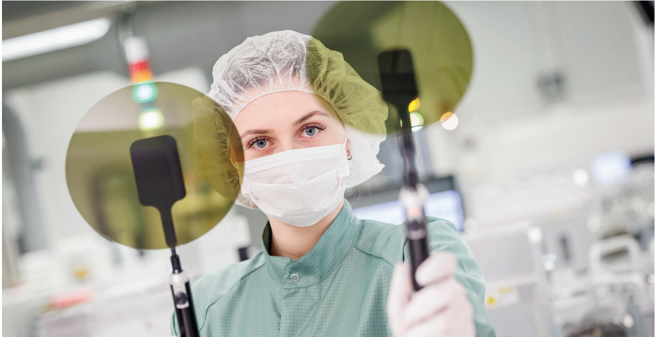
Epitaxy on SiC substrates with 150 mm and 200 mm diameter © Daniel Karmann / Fraunhofer IISB
