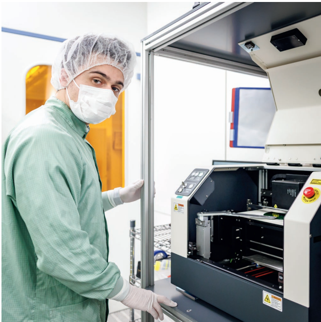
Carrier lifetime measurements on SiC epiwafers © Daniel Karmann / Fraunhofer IISB
