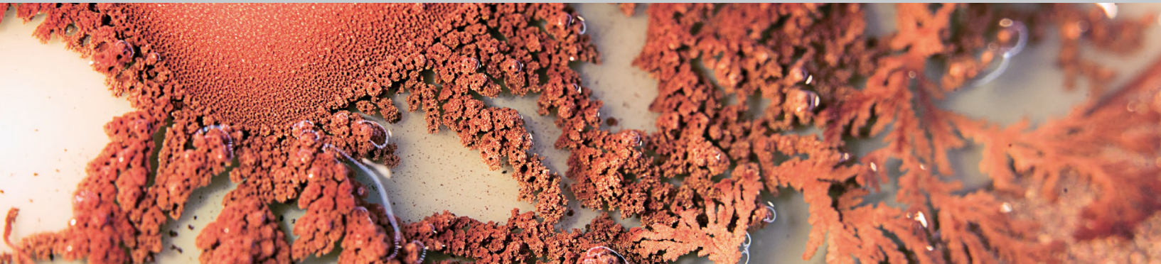
1 Dendrites on a ceramic circuit carrier
