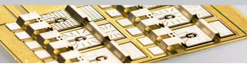
1 Double sided silver sintering of power semiconductors; design study of various top side ribbons for extended life time and processability
