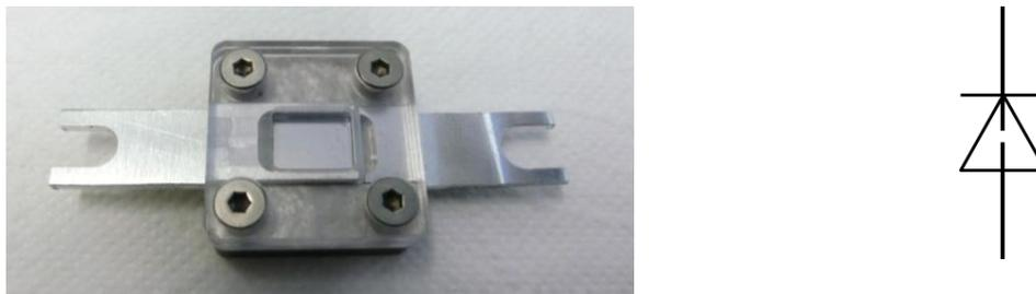
**Fig. 16: Assembled antifuse device with a top of polycarbonate for better visibility (source Fraunhofer IISB)**
