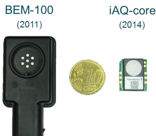
**Fig. 5: Evolution of gas sensor size over the project period**
