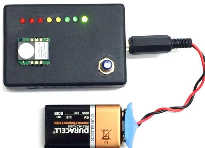
**Fig. 4: Gas Sensor evaluation kit**
