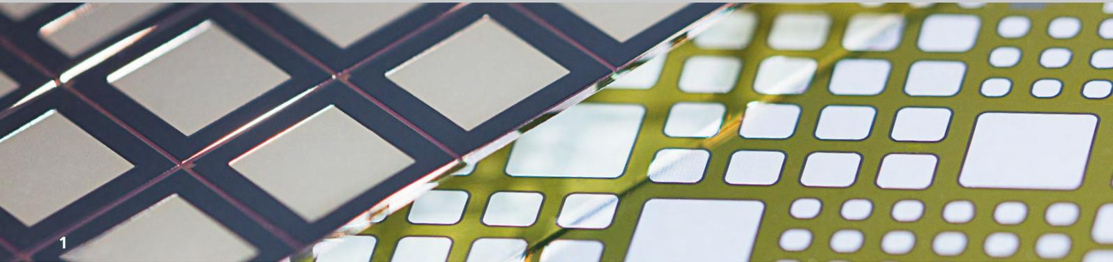
1 Processed SiC wafers featuring JBS-diodes with different device area and current-handling capability
