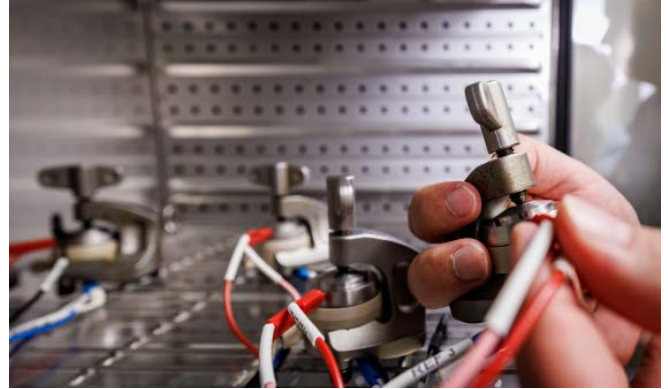
Electrochemical characterization of laboratory test cells in the climate chamber © Daniel Karmann / Fraunhofer IISB
