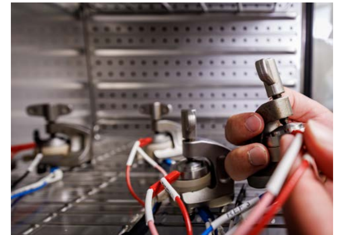
Electrochemical characterization of laboratory test cells in the climate chamber © Daniel Karmann / Fraunhofer IISB
