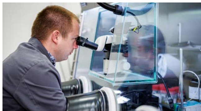
Post-mortem analysis of battery cells under inert conditions to investigate ageing mechanisms © Daniel Karmann / Fraunhofer IISB
