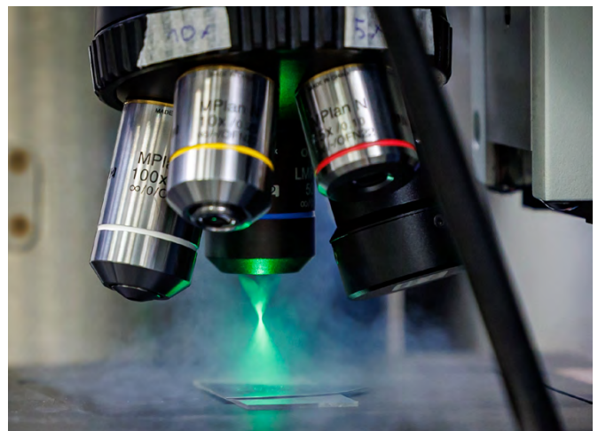
Confocal micro-Raman measurements providing both a high spatial and spectral resolution © Daniel Karmann / Fraunhofer IISB
