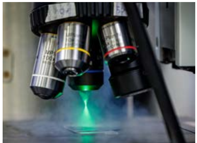
Confocal micro-Raman measurements providing both a high spatial and spectral resolution © Daniel Karmann / Fraunhofer IISB
