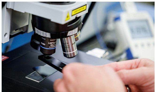
Assessing laser power at the objective lens © Daniel Karmann / Fraunhofer IISB
