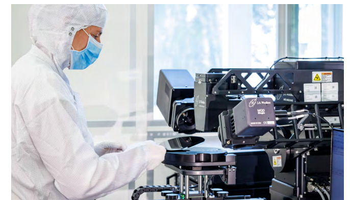
Optical characterization using a spectroscopic ellipsometer © Daniel Karmann / Fraunhofer IISB
