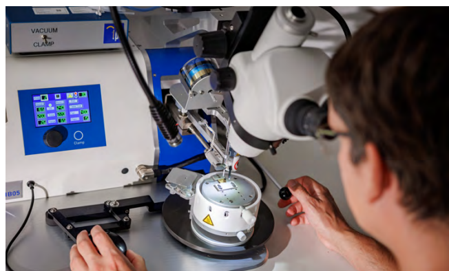
Device contacting via bonding wire © Daniel Karmann / Fraunhofer IISB
