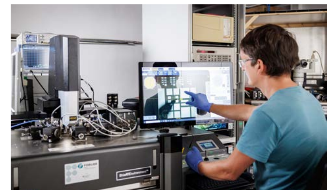
Electrical characterization at wafer probe station using parameter analyzer © Daniel Karmann / Fraunhofer IISB
