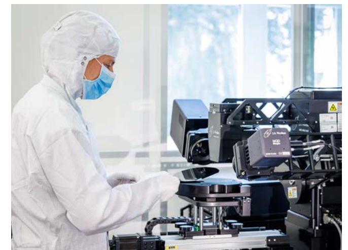
Optical characterization using a spectroscopic ellipsometer © Daniel Karmann / Fraunhofer IISB
