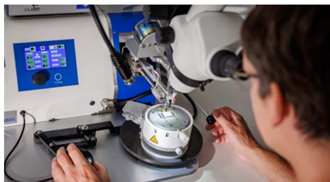
Device contacting via bonding wire © Daniel Karmann / Fraunhofer IISB
