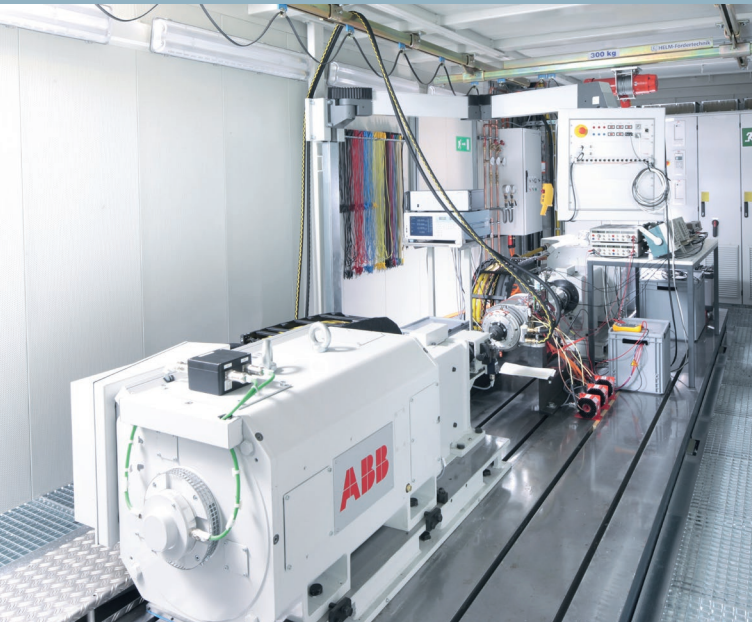
Test center for characterizing two motor axle drives © Kurt Fuchs / Fraunhofer IISB
