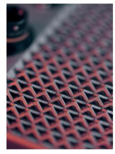
Additively manufactured cooling structure
