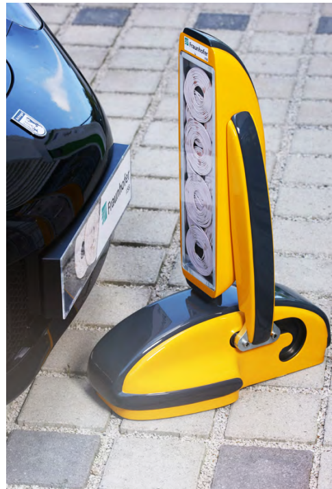
Primary and secondary unit of the vertically oriented IPT system developed by Fraunhofer IISB © Anja Grabinger / Fraunhofer IISB
