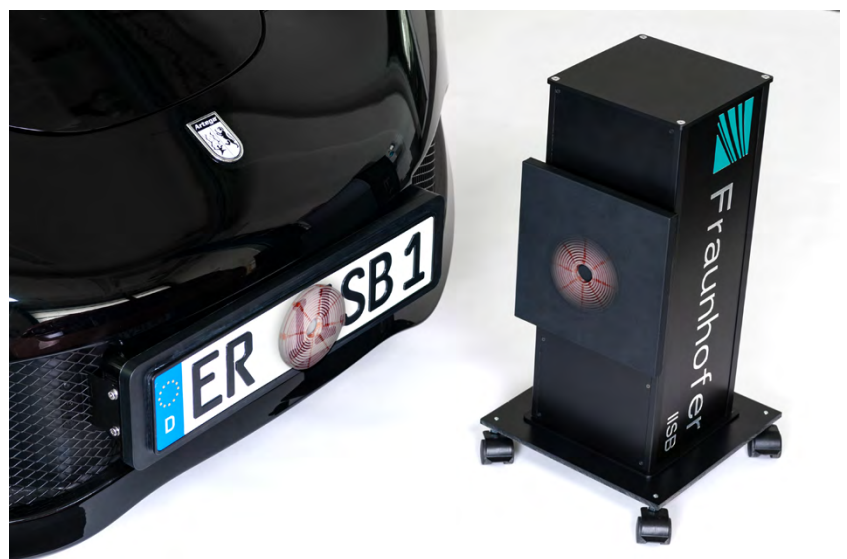
Primary and secondary unit of the vertically oriented IPT system developed by Fraunhofer IISB © Fraunhofer IISB
