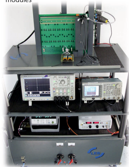
Fig. 2: Extremely low inductive (3nH) double pulse measurement setup
