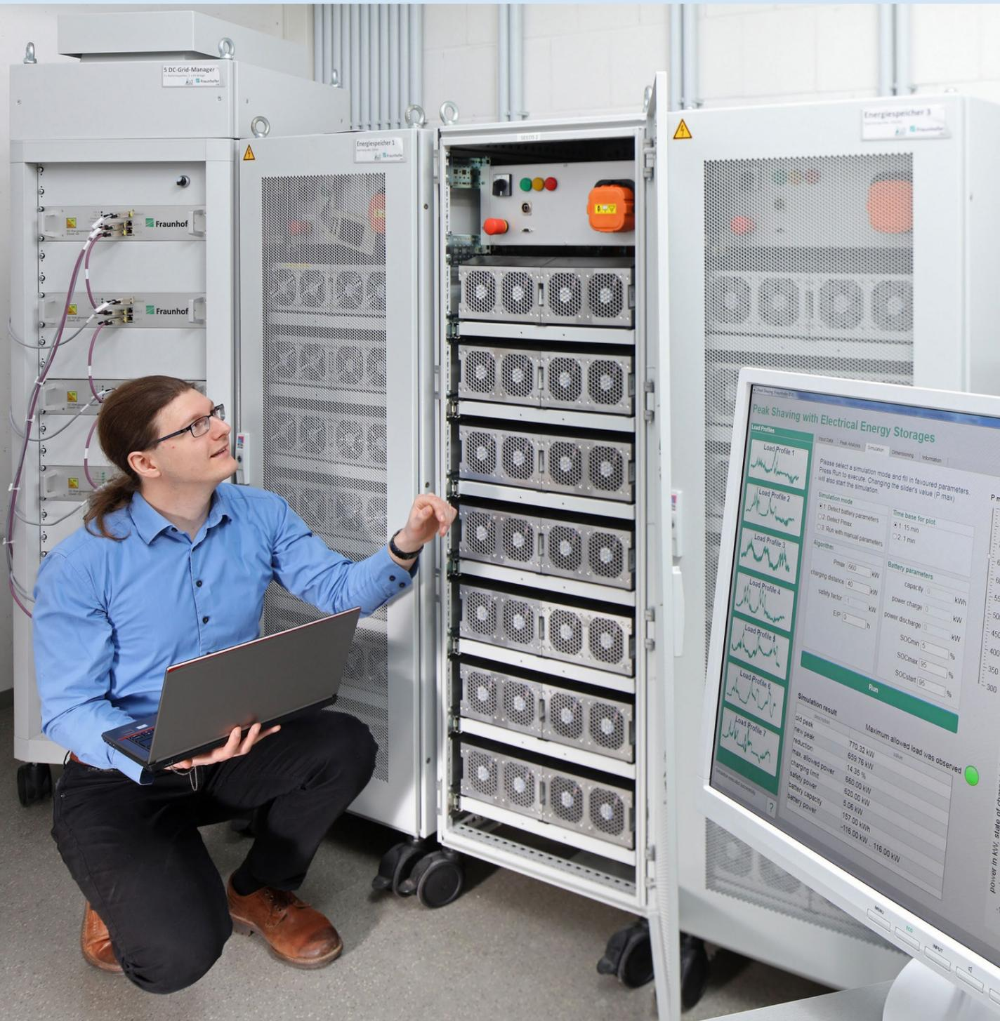
no risk that a peak could happen, the battery system can be charged. To avoid the generation of new peaks because of charging the electrical energy storage, a dead band (charging distance) is introduced. The resulting threshold is called charging limit.
