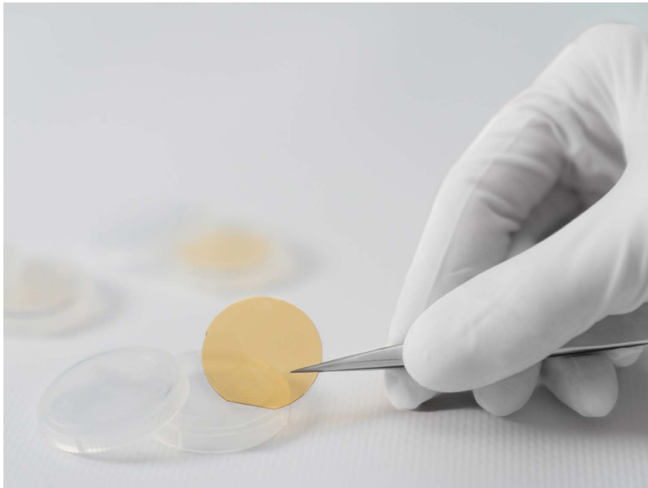
Epi-ready, single crystalline PVT-AlN-wafer fabricated at Fraunhofer IISB © Elisabeth Iglhaut / Fraunhofer IISB
