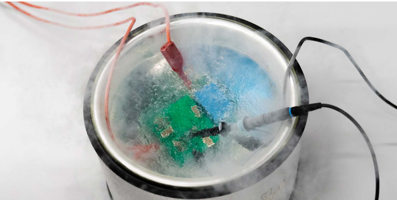
Electrical test of a cryogenic GaN inverter module in liquid nitrogen © Elisabeth Igthaut / Fraunhofer IISB
