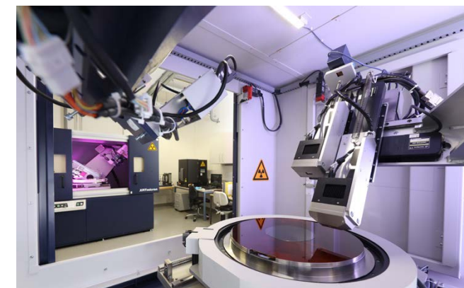
Fraunhofer IISB is a pioneer in the application of XRT for the dislocation quantification in SiC and continues to explore industrial use cases of this technique with its broad range of lab-scale XRT equipment © Kurt Fuchs / Fraunhofer IISB
