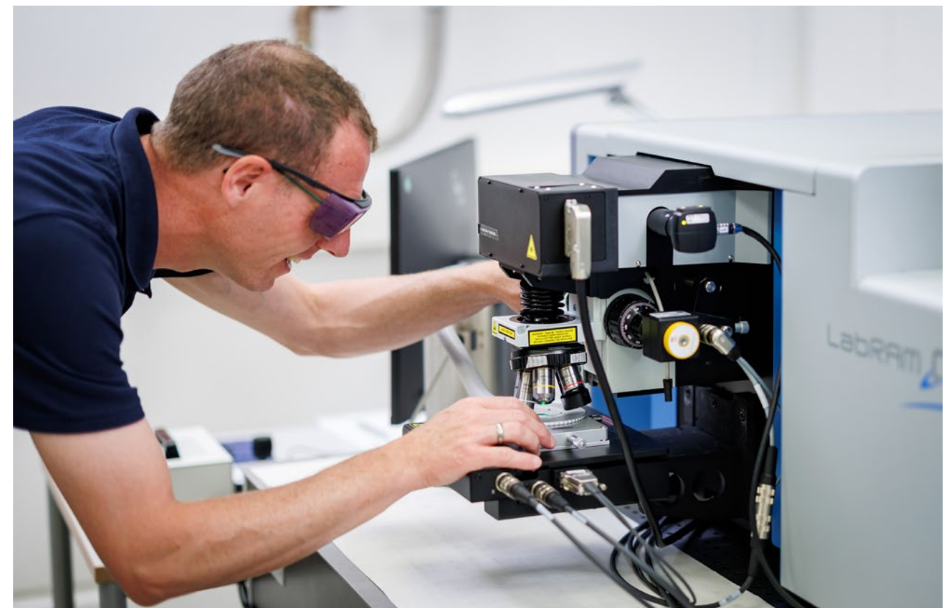
Material characterization at cryogenic temperatures (77 K) © Daniel Karmann / Fraunhofer IISB
