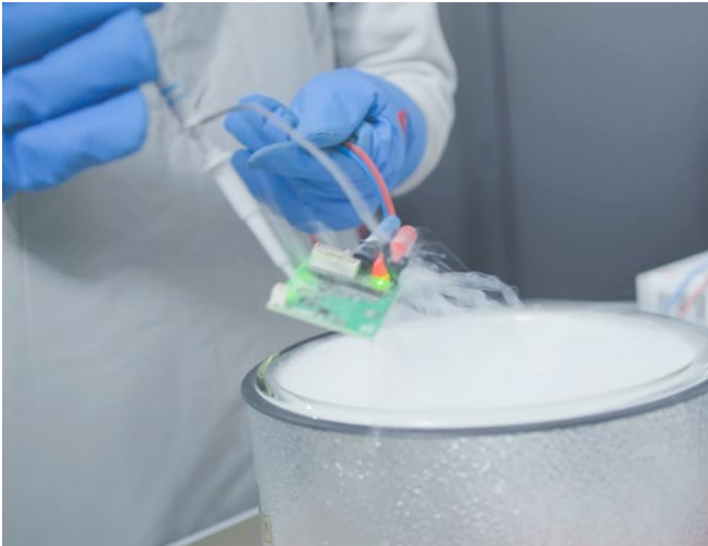
The IISB developed cryogenic cooled ultra-high-efficiency wide-bandgap power electronics cooled with liquid nitrogen © blubb.media / Fraunhofer IISB
