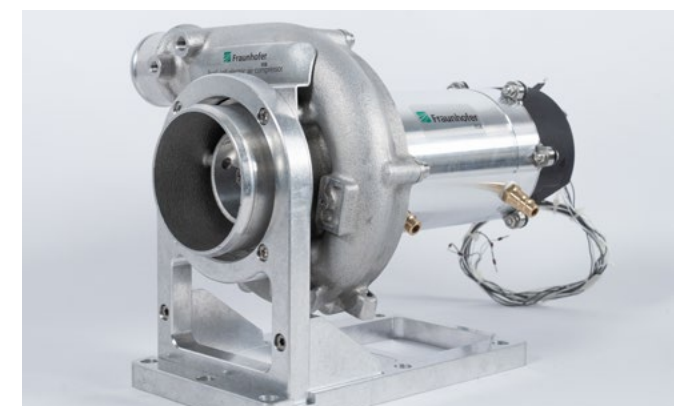
Highspeed drive for fuel-cell air compressors with 80 kW of peak power at 150,000 rpm, direct liquid cooling, three-stage GaN inverter and a power density of 30 kW / kg © Elisabeth Iglhaut / Fraunhofer IISB
