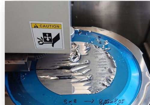
Delamination of back-end metallization during wafer dicing.
