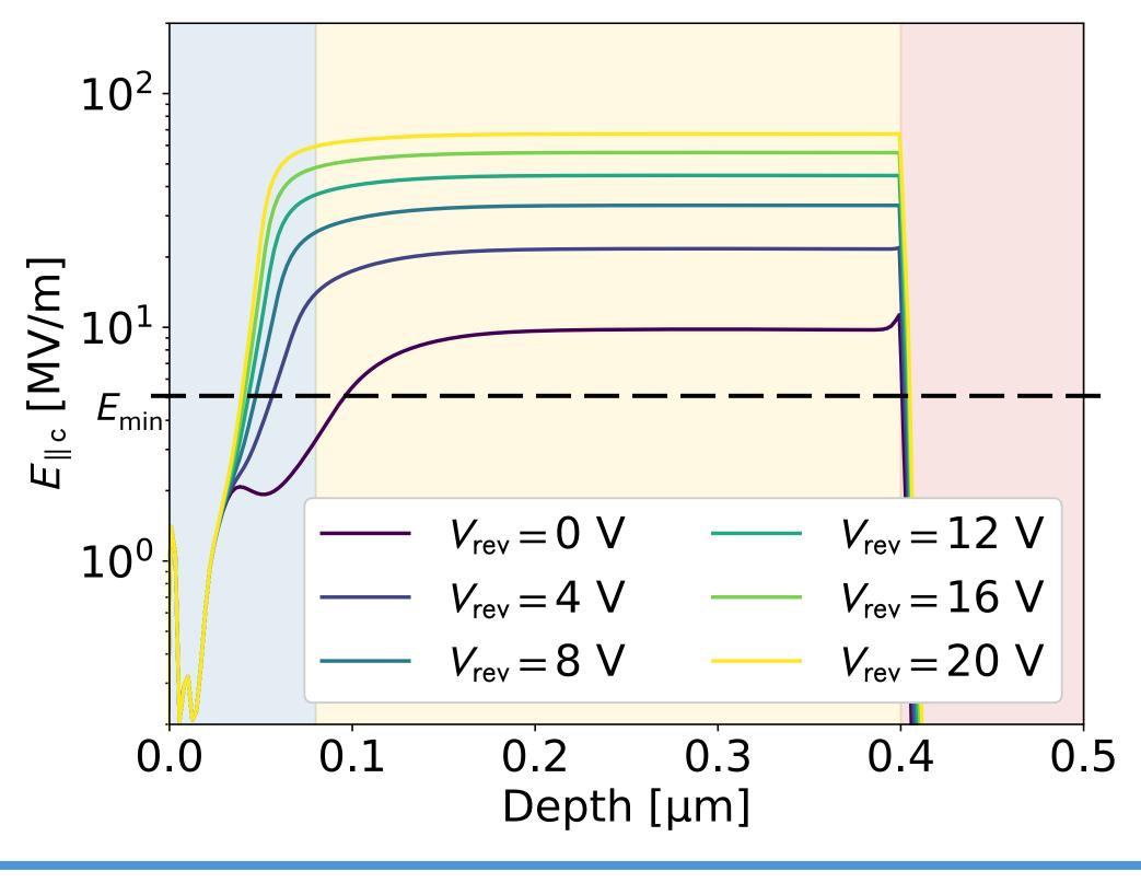
• In thermal equilibrium the intrinsic layer of the pin-diode offers a wide region to host V<sub>Si</sub> in optically active charge state (see green region below)
