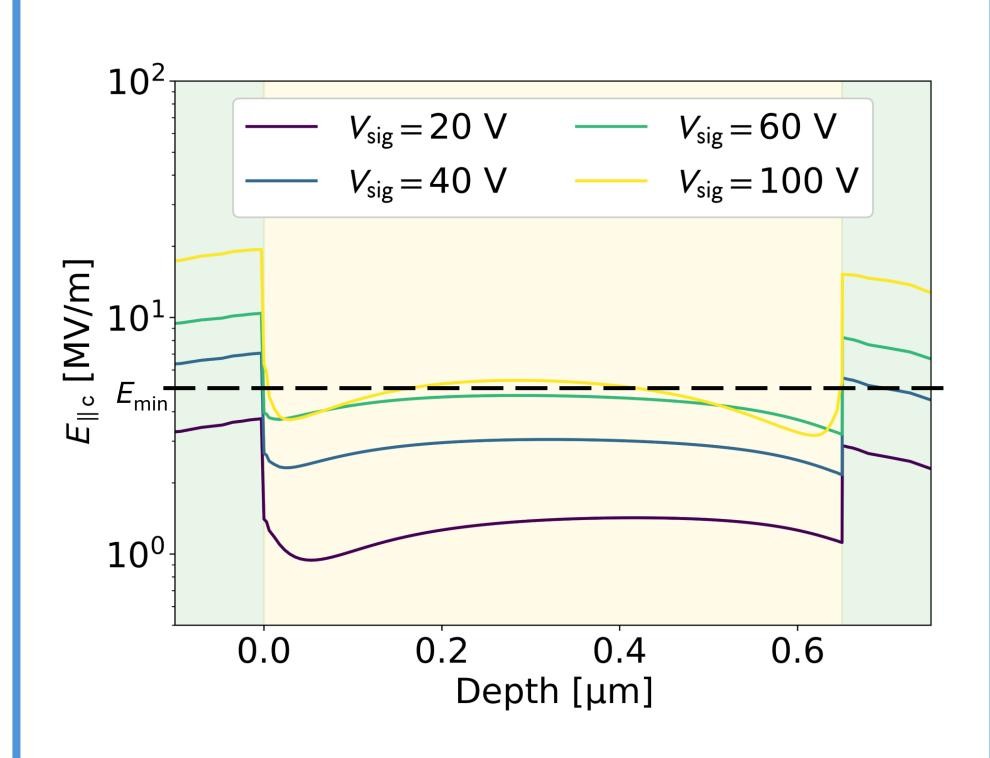
Maximum achievable electric field strength scales with waveguide height H and bandgap  $E_g$  due to **Fermi level** pinning at the interfaces
