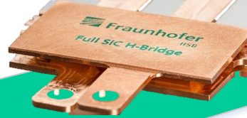
SiC- Chip on busbar
