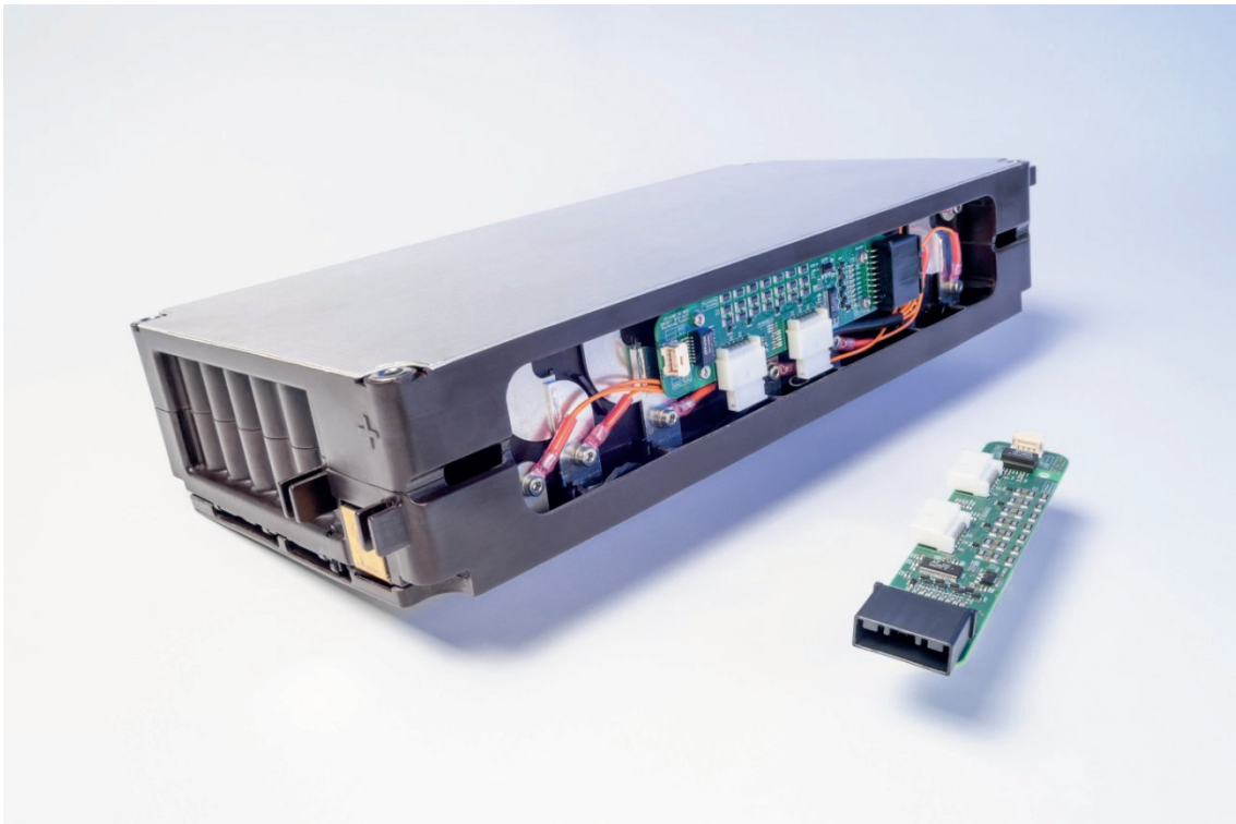
High energy density automotive battery module with cost-optimized battery monitoring electronics developed by Fraunhofer IISB with Dräxlmaier (Germany), Panasonic (Japan), and IFEVS (Italy). Picture: Fraunhofer IISB
