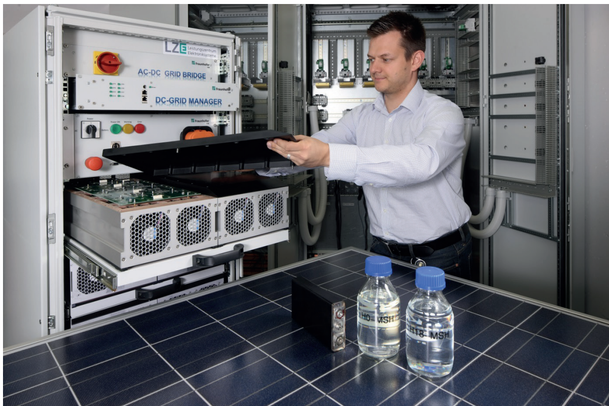
Within LZE, intelligent DC microgrids are integrated with lithium-ion systems for short-term storage of electrical energy, and with LOHC-based chemical systems for seasonal storage. (Photo: Kurt Fuchs / Fraunhofer)
