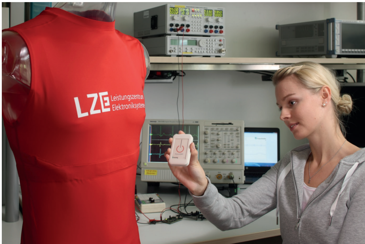
FitnessSHIRT (left) with integrated electrodes and a respiratory band to measure a single-channel-ECG and the respiratory rate. Measured data are collected on a technical unit (in model's hand; clipped on the back of the shirt during activity) and sent via Bluetooth to a smartphone or tablet. (Photo: Kurt Fuchs / Fraunhofer IIS)
