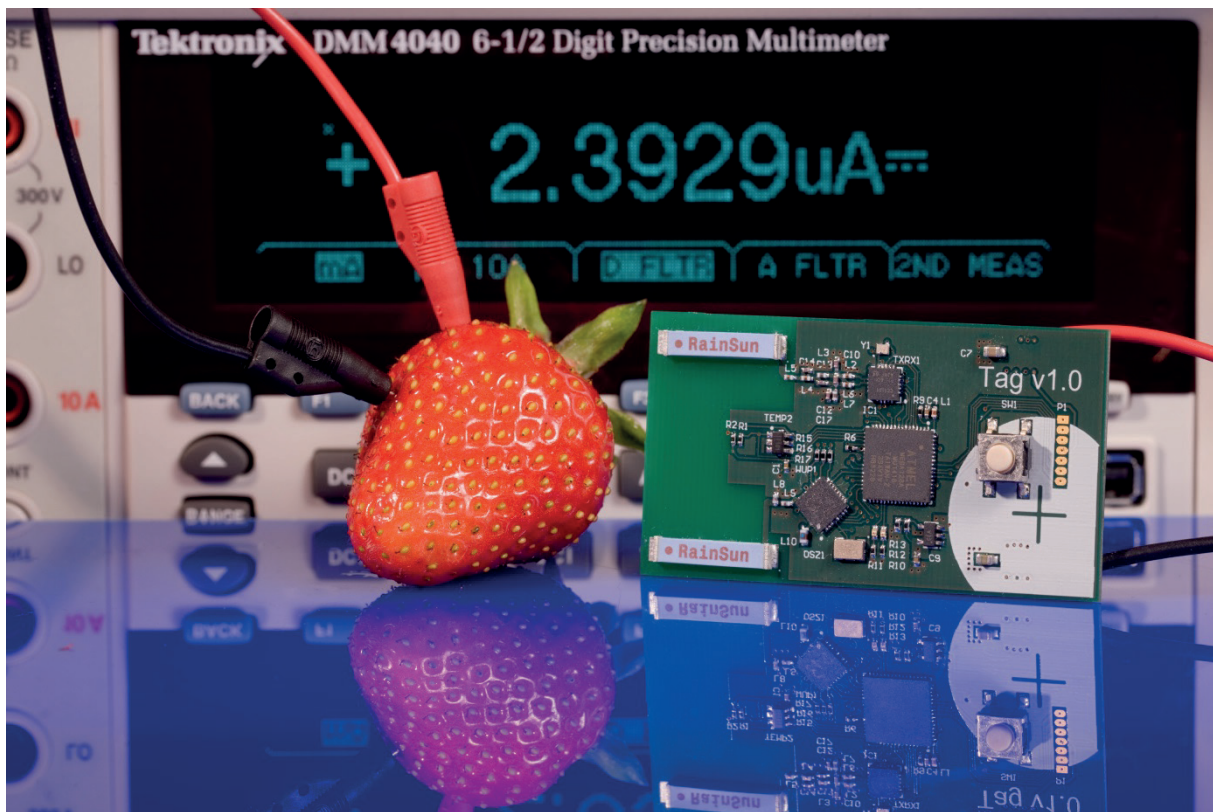
Wireless module containing wake-up receiver prototype with fruit power supply (Photo: Kurt Fuchs / Fraunhofer)
