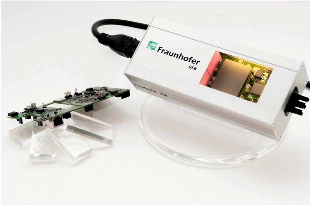
*Intelligent and data-connected DC-Power Supply by Fraunhofer IISB for monitoring and analysis of power quality and consumption. Picture: Fraunhofer IISB*
