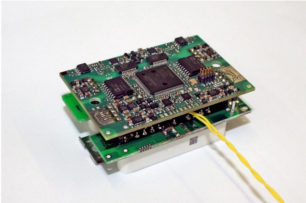
*Intelligent Power Unit by Fraunhofer IISB based on a novel 2-wire interface technology.
