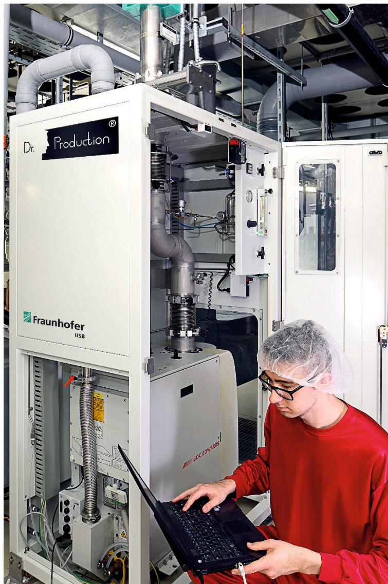
Vacuum system with 100% real-time facility state monitoring for deposition processes in semiconductor manufacturing. A machine-learning algorithm predicts the rest of useful life of the vacuum system until contamination gets critical. Picture: Kurt Fuchs / Fraunhofer IISB
